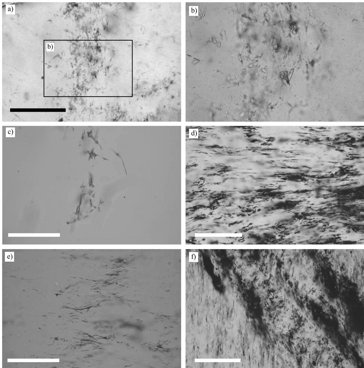
**Fig. 6.** Representative photomicrographs of distorted vesicle textures: **a)** and **b)** P10-1 (note **b** is located within **a**; scale bar = 250  $\mu\text{m}$ ); **c)** P2B-D (scale bar = 100  $\mu\text{m}$ ). Representative photomicrographs of stretched-distorted vesicle textures: **d)** P2B-N (scale bar = 200  $\mu\text{m}$ ); **e)** P2B-B (scale bar = 200  $\mu\text{m}$ ); **f)** P6B-B (scale bar = 300  $\mu\text{m}$ ).
