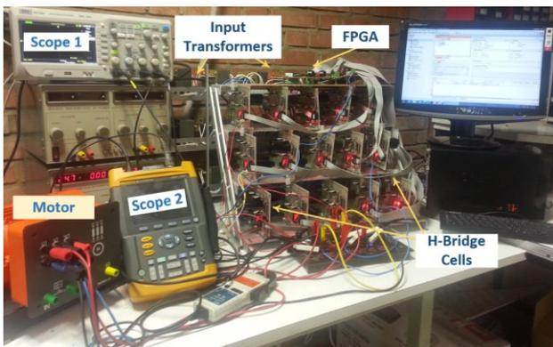
Fig. 12. Experimental setup: an 11-level CHB-MLI.
