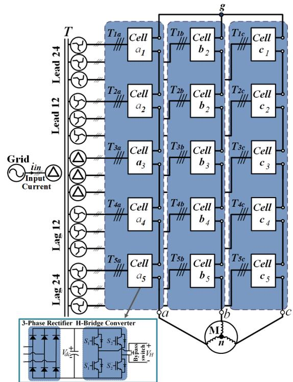
Fig. 1. An 11-level Cascaded H-bridge Multilevel Inverter.
