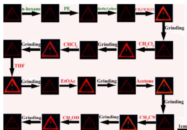
**Fig. 5** Photographic images under illumination with UV light of the monitoring of VOCs by **1** after exposure to different VOCs and grinding.
