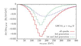
**Figure 8.** Contributions of the first two generations and the third generation to the interference in  $gg \to W^+W^-$  at leading order in perturbative QCD.
