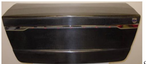
Fig. 11 Structural supercapacitor flat laminate (a); model car body (b) and trunk lid with added chrome trimming and lit LED lights (c).
