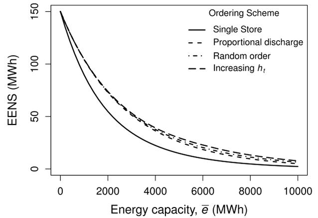
**Fig. 5.** EENS versus  $\bar{e}_{tot}$  for scenario 3 and single store with same capacities – real-time decisions, various coordination strategies. The curve for the ‘decreasing  $h_t$ ’ method is omitted since it is indistinguishable from the ‘proportional’ method curve.
