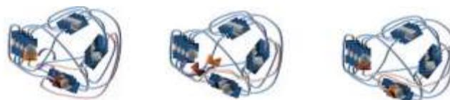
**Fig. 22** Proposed optical healing of a metallosupramolecular, phase-separated network (reproduced with permission from ref. 48).
