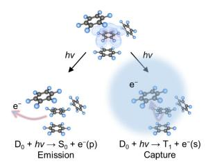
**Figure 3.** Schematic of electron capture mechanism that gives rise to the low-energy electrons observed in Figure 1. Photoemission from  $C_6F_6^-$  in the cluster can lead to p-wave emission or s-wave emission, depending on the detachment channel. Only s-wave emission can lead to electron capture via a non-valence state of the cluster.
