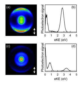
**Figure 2.** A raw photoelectron image (a) and spectrum (b) of  $C_6F_6^-$  taken at hv = 4.3 eV, and at hv = 5.0 eV in (c) and (d), respectively. The images indicate the representative photoelectron angular distribution of the different direct detachment channels. The polarization axis is indicated as the double arrow.
