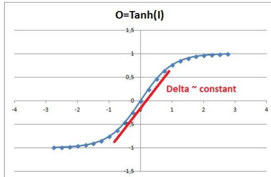
Figure 9: Plot of the hyperbolic transfer function
