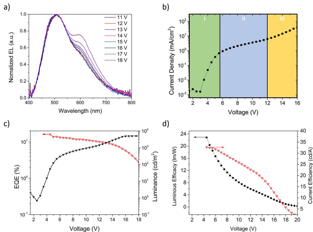
**Figure 5.** Orange-green-blue study of a device containing the optimised structure for a W-OLED. **(a)** EL spectra at different voltages. **(b)** Current density-voltage (JV) with three different regimes: I the space charge limited current (SCLC); II and III the different carrier balance regimes. **(c)**  $\eta_{\text{ext}}$  and luminance dependences with voltage and **(d)** Luminous and current efficiencies of the device.
