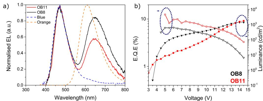
**Figure 3.** Study of the concentration of POZ-DBPHZ in an orange-blue structure with relative concentrations of orange of 8% and 11%. **(a)** Electroluminescence (EL) spectra of both devices together with the EL of each material independently, taken from<sup>36,37</sup>. **(b)** Electrical performance of the devices used for both structures.
