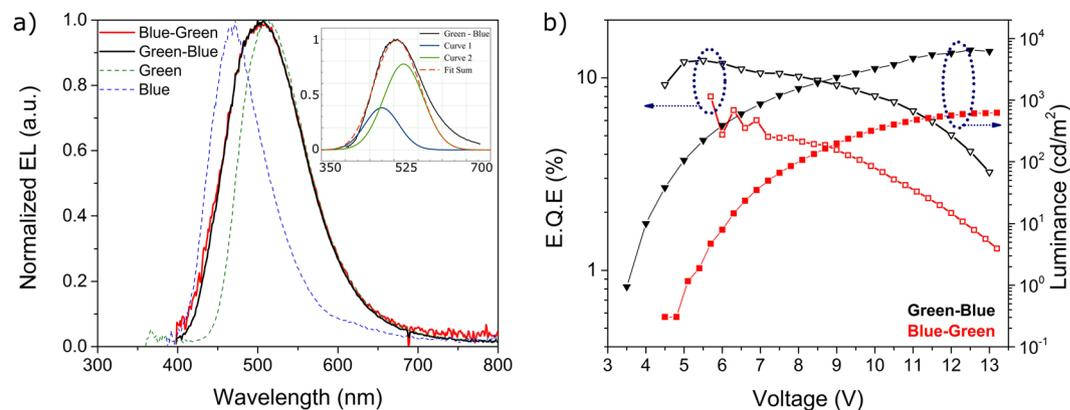
**Figure 2.** Study of the orientation of the layers in a green-blue structure. **(a)** Electroluminescence (EL) spectra of both devices together with the EL of each material independently, taken from<sup>31,32</sup>. The inset shows the deconvolution of the EL spectrum of the green-blue structure. **(b)** Electrical performance of the devices used for both structures.
