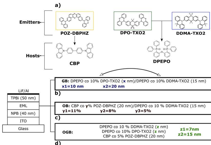
**Figure 1.** (a) Molecular structures of host and guest molecules used as emitting layers in a general device structure (Tables S1–3). Three studies were conducted: (b) one with green and blue emitters with thickness (x) of the green's Host-Guest system between 10 and 20 nm, (c) another with orange (concentrations – y – of 5, 8 and 11%) and blue. The best results were merged into the final device structure (d) and thicknesses of DPEPO (z) were varied between 7 and 15 nm.
