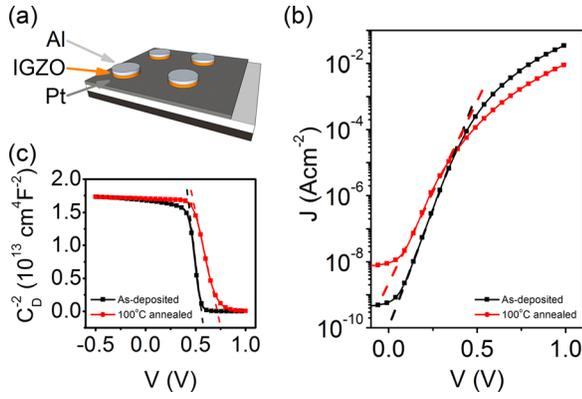
FIG. 1. (a) Schematic of the Pt-IGZO Schottky diodes. (b) J-V characteristics of the Schottky diode. (c)  $1/C^2$  curve as a function of voltage. The slope gives the built-in voltage  $V_{bi}$  and the background doping density  $N_{bg}$ .
