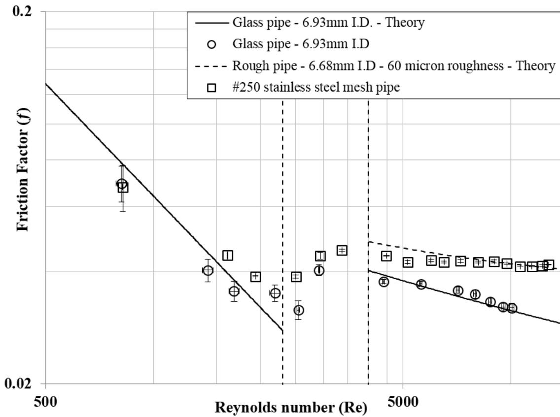
Figure 4. The friction factor ( $C_D$ ) at different Reynolds number ( $Re$ ) for a theoretical glass pipe (—), an experimental glass pipe (○), a theoretical pipe with 60 micron roughness (- - -), and a #250 stainless steel mesh pipe (□).
