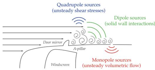
**Figure 4.** Aeroacoustic sources in the sideglass region, adapted<sup>27</sup>
