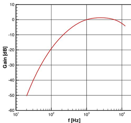
**Figure 3.** Frequency response of the A-weighted filter
