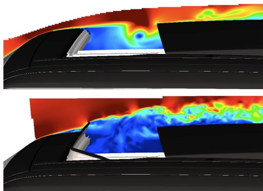
**Figure 7.** Open sunroof contours of transient velocity magnitude: (top) deflector removed, (bottom) mesh deflector<sup>78</sup>
