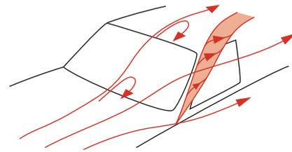
**Figure 5.** Typical vortex structure around the A-pillar, adapted<sup>24,38</sup>
