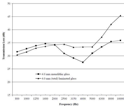
**Figure 6.** Comparison of the transmission loss of monolithic and laminated glass windows with the same total thickness, adapted<sup>63</sup>
