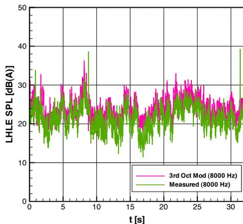
**Figure 8.** Comparison of simulated and measured cabin noise using a modulation approach<sup>96:109</sup>
