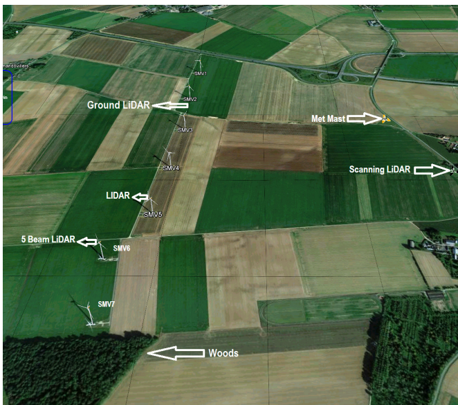
Fig. 1: SMV layout and surrounding with positions of met mast and LiDARs [26]
