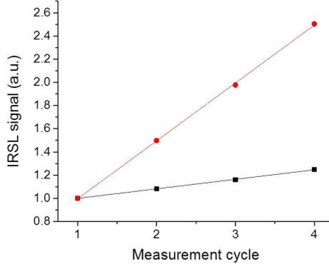
Figure 3: Change in IRSL response with repeated cycles of  $\beta$  irradiation (6 Gy) where the IRSL measurement was performed at a sample temperature of 70 °C and in an atmosphere of air (filled squares) or nitrogen (filled circles). Detection window: BG-39.
