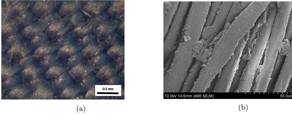
Figure 1: a) Image of a piece of blue polyester-mix fabric (F#3) showing the woven structure and filaments within each thread; b) Blue polyester-mix (F#3) showing filaments (x900 magnification)
