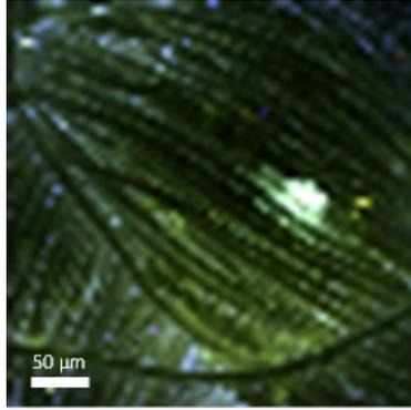
Figure 2: Cathodoluminescence (CL) images of the blue polyester-mix fabric with a blue spectral window (470 nm central wavelength,  $\delta= 100$  nm). Electron beam voltage, 10 keV.
