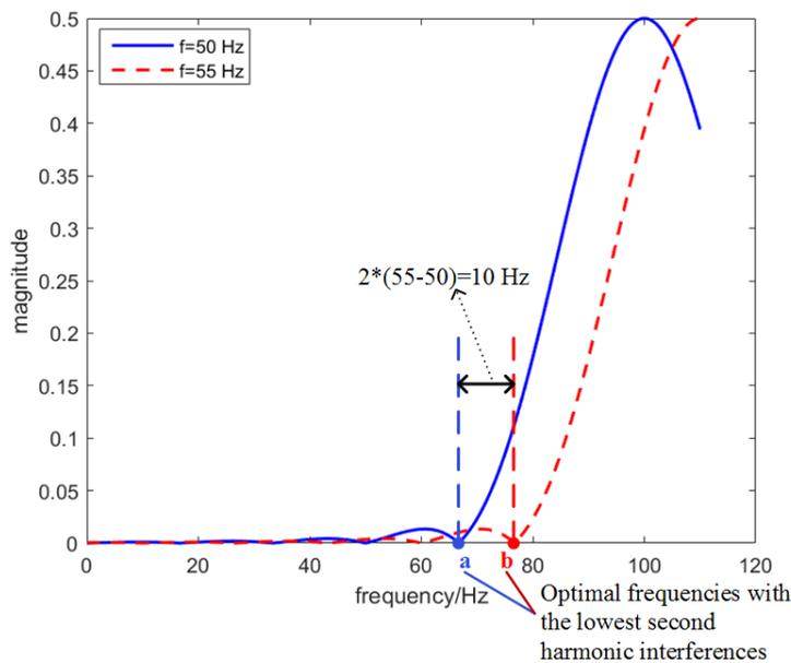
Figure 2. Illustration of the second harmonic interference. The red and blue lines are second harmonic interferences at different frequencies. The image second harmonic component is ignored. Only one bin used in the  $IpD^2FT$  is illustrated.
