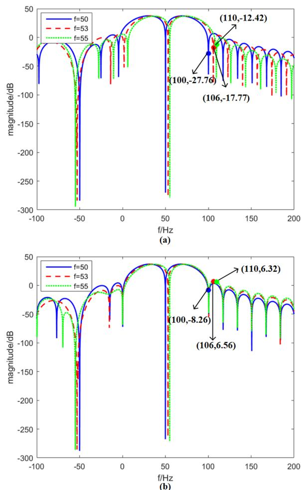
**Figure 4.** Instantaneous frequency response of the  $\text{e-IpD}^2\text{FT}$  and  $\text{IpD}^2\text{FT}$  for  $p_1$  estimation. The three-cycle Hanning window is chosen for illustration.  $f$  is set at 50, 53 and 55 Hz, respectively: (a)  $\text{e-IpD}^2\text{FT}$ ; and (b)  $\text{IpD}^2\text{FT}$ .
