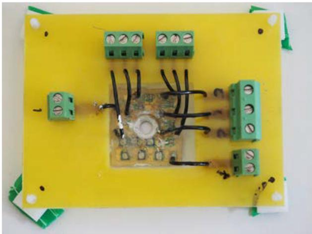
Fig. 4 SEMIKRON 01NAC066V3 MiniSKiiP module modified for testing
