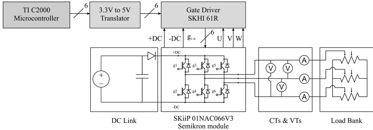
Fig. 3 Electrical circuit diagram of the experimental rig
