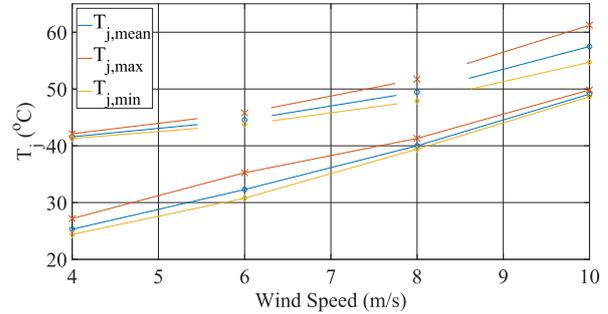
Figure 6:  $T_j$  results for equivalent wind speed tests. Dashed lines are simulated results and solid lines and experimental results.
