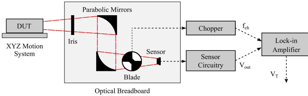
Figure 1: Experimental optical set-up.  $V_T$  is the temperature dependent voltage output and  $f_{ch}$  is the chopping frequency.
