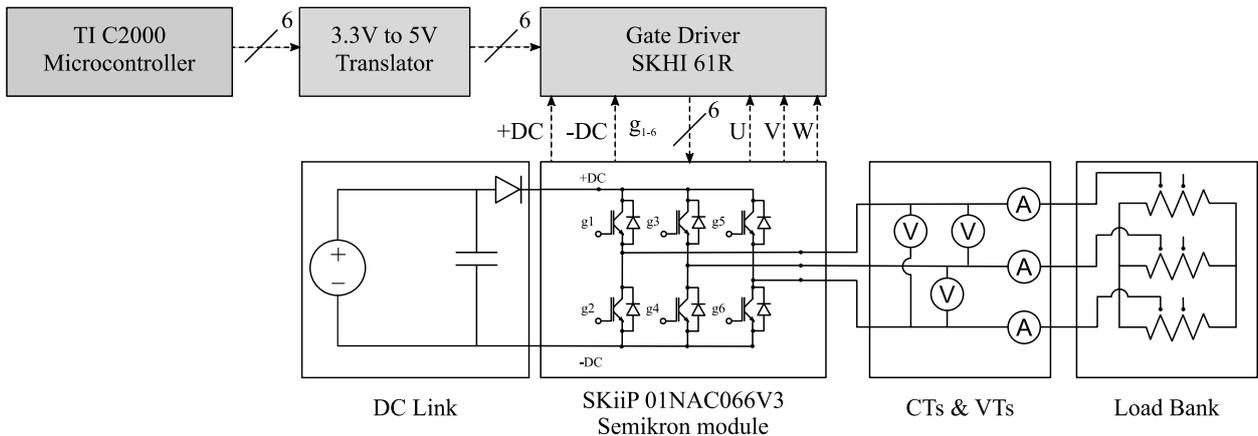
Figure 3: Electrical circuit diagram of the experimental rig.
