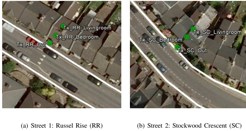
Fig. 1. Transmitter locations and route of the portable receiver (©Bluesky International Ltd, 2013)
