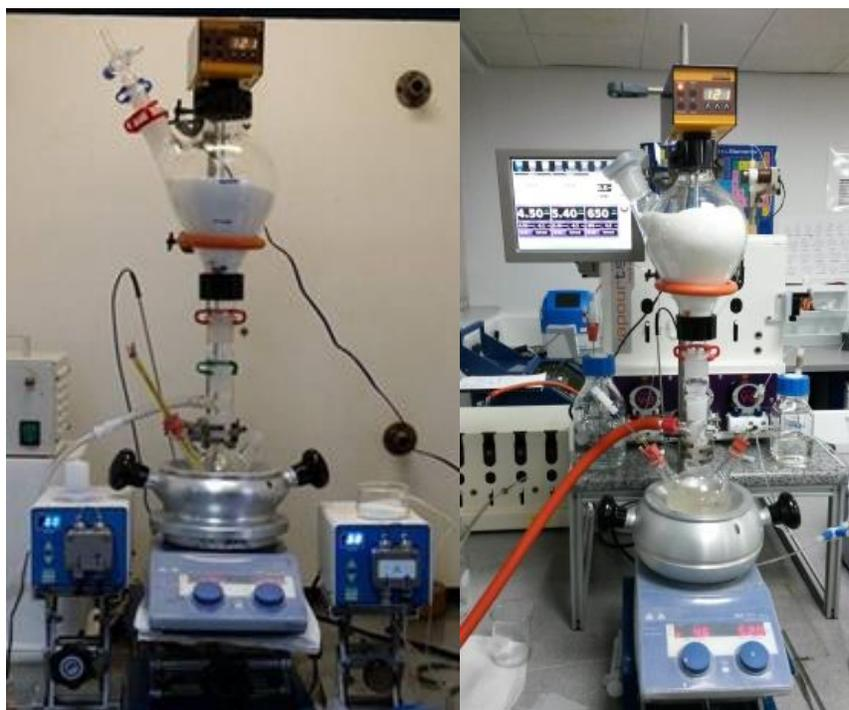
**Figure 3.** a) Prototype CSTR set-up for acylation of *D*-glucono-1,5-lactone (**2**) with HPLC pumps b) System coupled with the peristaltic pumps of the Vapourtec E series system.
