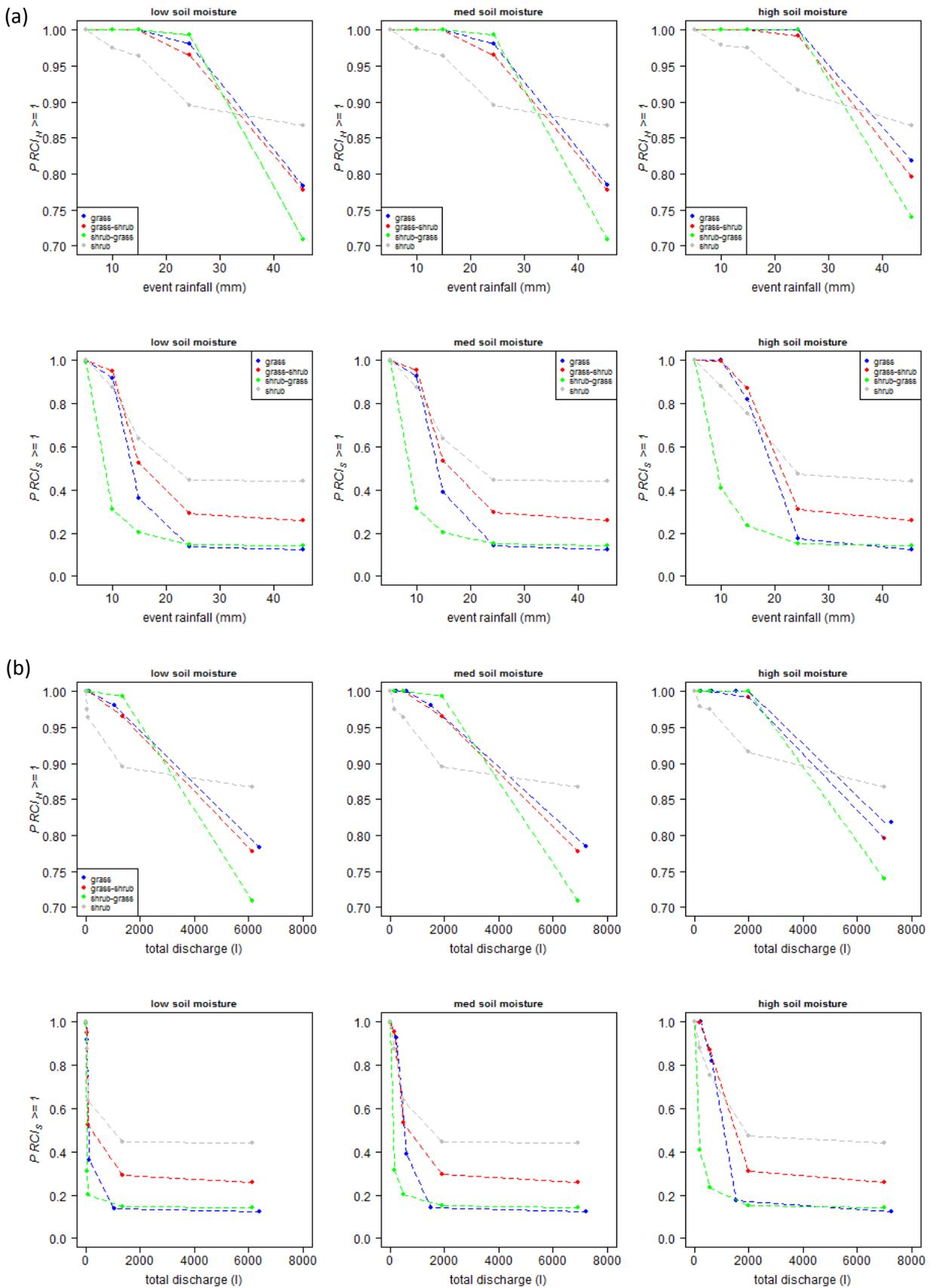
**Figure 7.** Percentile value ( $P$ ) at which  $RCI_H$  and  $RCI_S$  are  $\geq 1$  (i.e. connected) for (a) the different sized rainfall events and (b) the associated total discharge generated at the lower boundary of the study domain, plotted for low, medium and high soil-moisture content.
