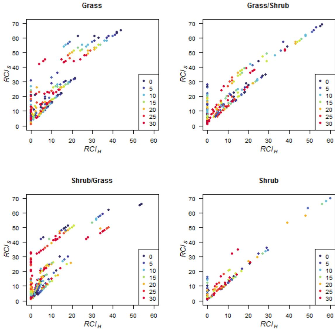
**Figure 6.** Relation between  $RCI_H$  and  $RCI_S$  for the 45 mm rainfall event for high antecedent soil-moisture content. Points are shaded according to distance (m) from the lower boundary of the study domain.
