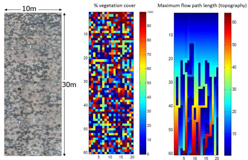
**Figure 1.** Aerial imagery used to calculate % vegetation cover (left); resulting % vegetation cover map (centre); and topographically defined maximum flow path length (no. cells; right).
