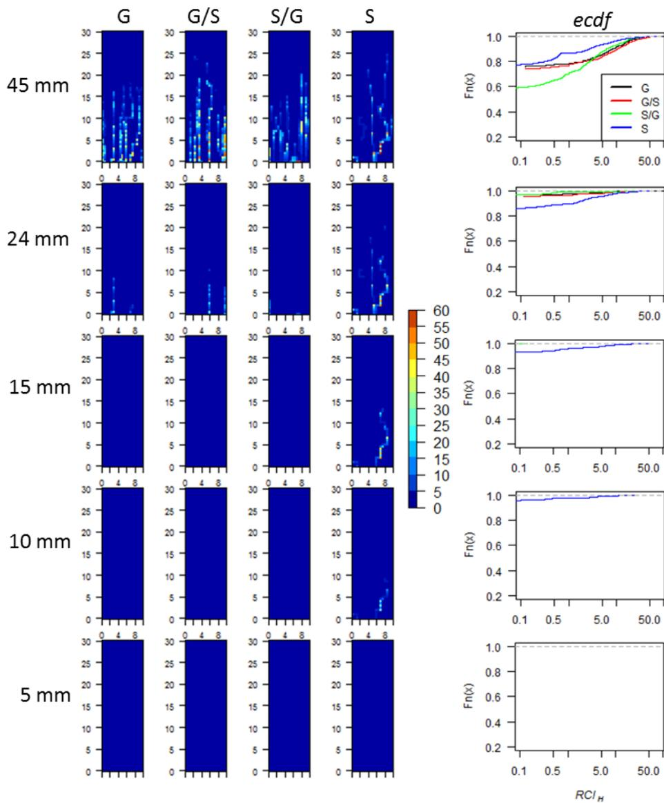
**Figure 4.** Spatial plots of  $RCI_H$  for different total rainfall event size (45 mm, 24 mm, 15 mm, 10 mm and 5 mm), for high soil-moisture content (left) and associated empirical cumulative distribution function of spatial  $RCI_H$  values (right).
