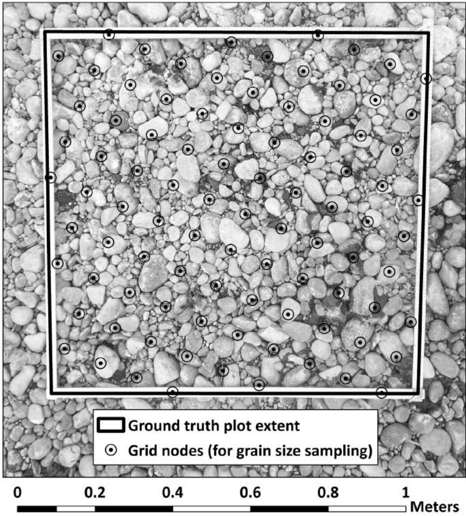
Figure 3. Example of a ground truth sample plot.
