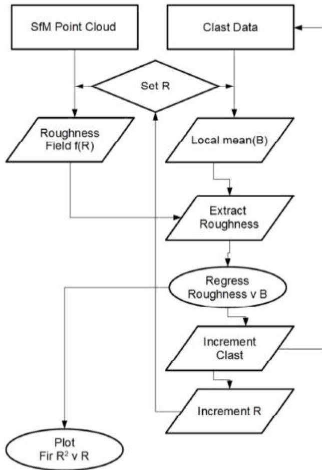
Figure 6. Roughness method, as applied to dense point clouds.  $K$  = radius size of spherical roughness kernel.
