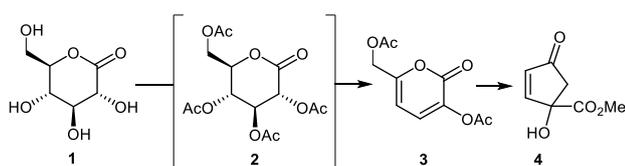
**Scheme 1:** Continuous flow synthesis of cyclopentenone **4**.
