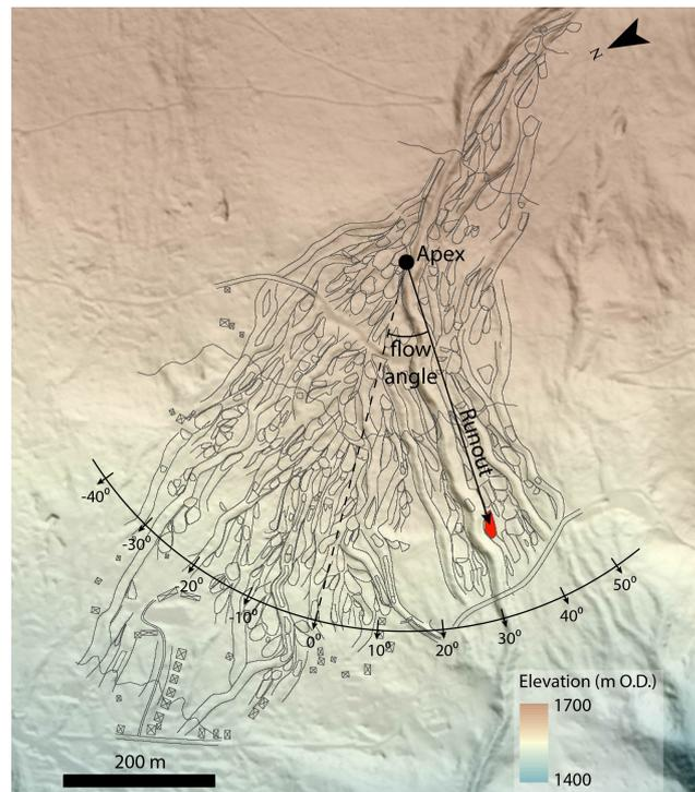
Figure 2: Method for pattern extraction and fan gradient calculation. Red polygon shows a debris-flow lobe deposit. Depositional patterns over time are quantified by the runout distance and flow angle from the fan apex. Average fan slopes are calculated per radial angle at multiples of 100 m from the fan apex. Grey outline marks the mapped debris-flow channels and deposits from [Stoffel *et al.*, 2008].
