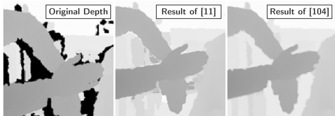
Fig. 14: Example of the result of [104] compared to [11]. Each hole is filled based on the distribution of its neighboring pixels [104] (reproduced from [11]).
