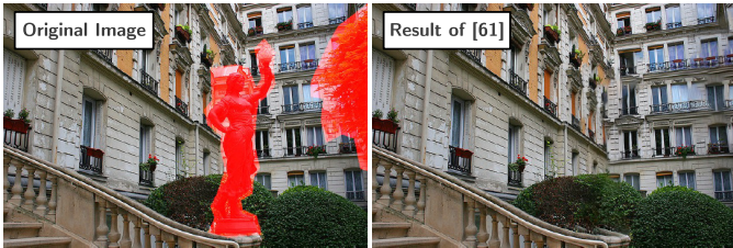
Fig. 6: Results of [61], achieved by adding the mid-level scene understanding constraints of translational regularity (via scale-invariant feature (SIFT) matching [72]) and planar perspective to guide the process (reproduced from [61]).
