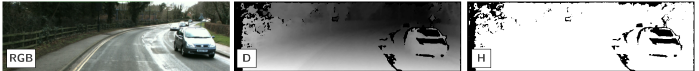
Fig. 1: Example of depth acquired via stereo correspondence in an urban driving scenario. Note the missing depth values despite accurate camera calibration.
