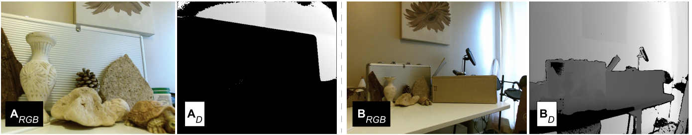
Fig. 9: Examples representing challenges involving depth textures (captured using Microsoft Kinect v2). When captured from close proximity, depth values of highly textured objects are missing due to the short camera distance (left). The same objects captured from a distance are smooth with little granular relief (right).
