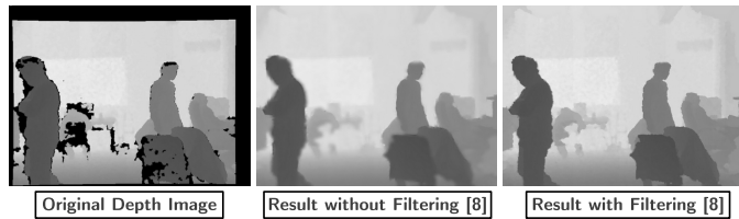
Fig. 21: Results of depth inpainting [8]. The approach is an improved fast marching-based [41] method guided by the color image (reproduced from [8]).
