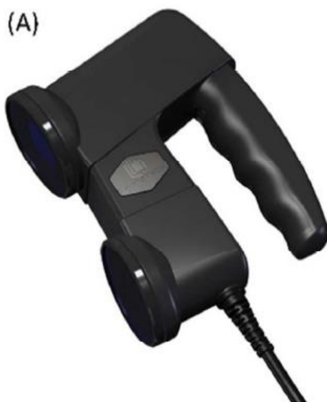
Figure 4. (A) The Mantis Vision F5 Short Range Hand-held Imager (OR3D, 2015); (B) Use of the Hhl on a bare peat plot.
