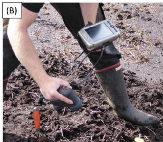
Figure 4. (A) The Mantis Vision F5 Short Range Hand-held Imager (OR3D, 2015); (B) Use of the Hhl on a bare peat plot.
