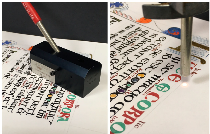
Fig. 3 Reflectance spectrometer based upon that published by Aceto et al. using a fibre probe to investigate a model manuscript surface, left , using sample block to ensure constant distance from the surface, in 45° geometry, and right , clamped 8mm above page in perpendicular geometry.
