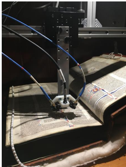
Figure 2, ‘Team-Pigment’ FORS probe, left , showing head suspended from the gantry and the vertical adjustment system, right , the alignment of the two spots on a test sheet of blue paint. The single bright spot in the centre demonstrates the correct vertical alignment of the head for optimum collection efficiency.
