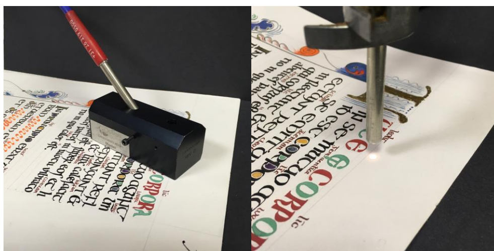
Figure 3. Reflectance spectrometer based upon that published by Aceto et al , using a fibre probe to investigate a model manuscript surface, left , using sample block to ensure constant
