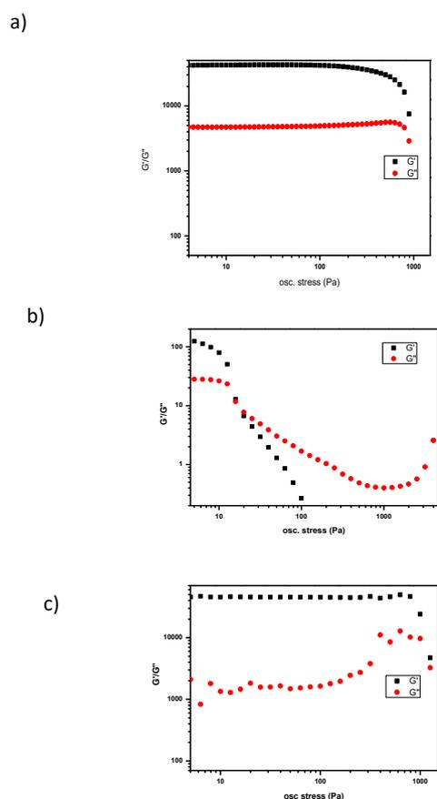
**Figure 4.** Stress sweep experiments at a concentration of 2% wt. for a) **4a** in 1,4-butanediol ( $\sigma = 914$  Pa). b) **4d** in DMF ( $\sigma = 20$  Pa). c) **4e** in 1,4-butanediol ( $\sigma = 1585$  Pa).
