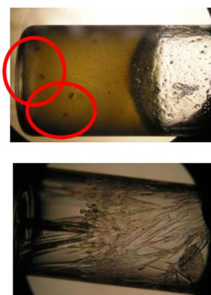
**Figure 8.** Crystals of niflumic acid grown inside the gel of **4e** (top) in methanol and by solution evaporation (bottom).
