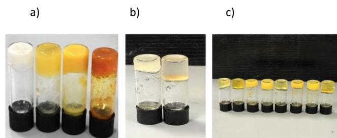
**Figure 1.** a) Gels of **4a** at 2% wt. in (from left to right) 1,4-butanediol, 2-propanol, 1-pentanol and methanol. b) Gels of **4d** at 2% wt. in (from left to right) DMF and diethylene glycol. c) Gels of **4e** at 1% wt. in (from left to right) in ethanol, methanol, hexane, 2-butanol, 1-propanol, 1-butanol, 2-propanol and 1,4-butanediol.
