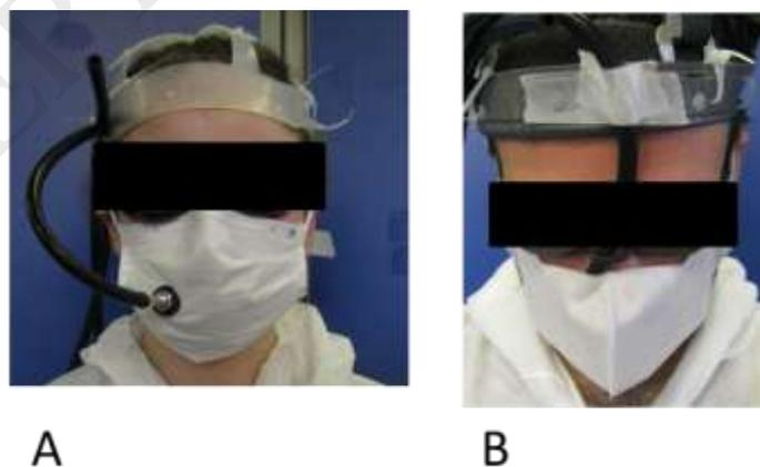
**Figure 2:** Attachment of sampling tube and probe A) PM<sub>2.5</sub> Surgical (J) as an example for all masks except B) Basic flat-fold (I) mask which had a slightly different arrangement for the measuring tube
