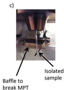
**Figure 1. a) Photograph of apparatus used highlighting i) standard MPT holder, ii) modified sample holder and iii) rubber stopper used to further hold shortened MPT in place. b) schematic of modified probe sample holder with dimensions and c) relative sample and baffle positions that facilitate sample release.**
