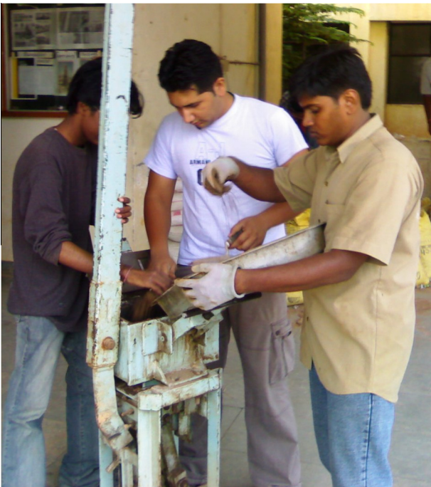
Plate 2. Transferring of wet mix into the block making mould of ASTRAM press.
