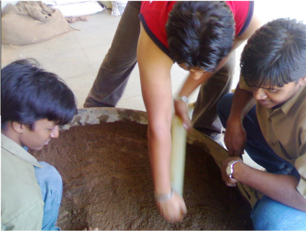
Plate 1. View showing wet mixing of ingredients used for the preparation of the blocks.
