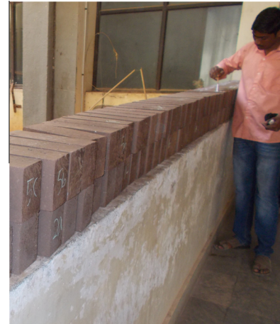
Plate 3. View of CSEBs being numbered for future identification.
