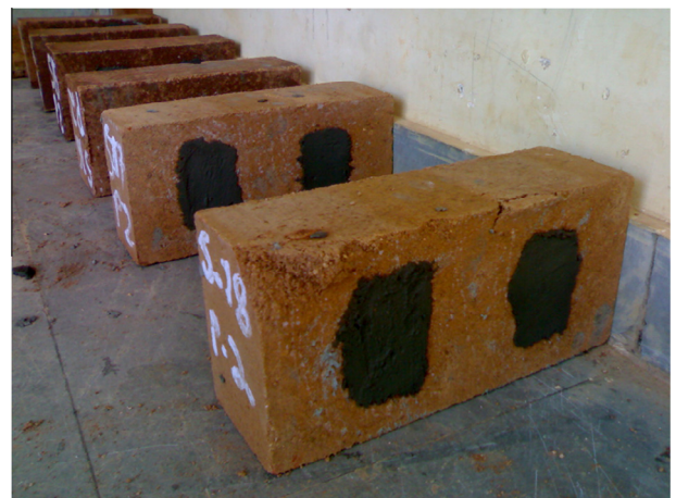
Plate 4. View showing frogs marks of CSEBs filled with 1:1 cement mortar.
