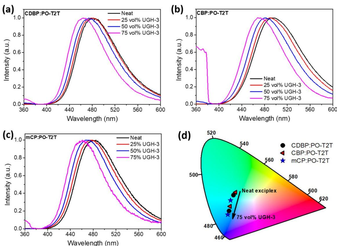
**Figure 2** Photoluminescence spectra of (a) CDBP:PO-T2T (b) CBP:PO-T2T and (c) mCP:PO-T2T exciplex films (D:A ratio 1:1) in different vol% of UGH-3 (d) 1931 CIE chromaticity diagram schematically showing the blueshift of the electroluminescence emission coordinates with increasing % vol% UGH-3 in all materials.
