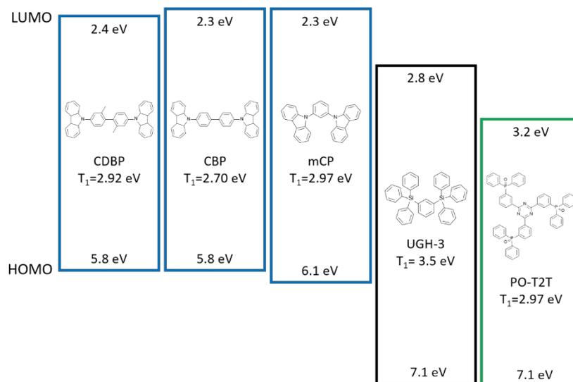
**Figure 1** Molecular structures and HOMO, LUMO and  $T_1$  energy levels of the exciplex forming donors (CDBP, CBP and mCP), acceptor (PO-T2T<sup>12</sup>) and the host used to dilute the exciplexes (UGH-3<sup>8</sup>).
