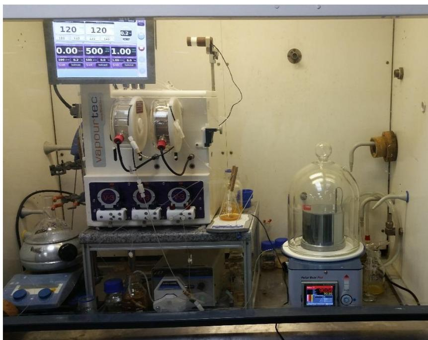
Figure S2 – Configuration of the Vapourtec and Polar Bear flow reactors for the synthesis of methyl coumalate.
