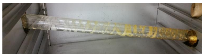
Figure 6. The helix effect seen as the reaction is occurring on the inner surface of the work-tube. The colour change from colourless to yellow can be seen as the reaction occurs. The opacity of the solution appears to change; this is due to the formation of gas bubbles which are escaping.
