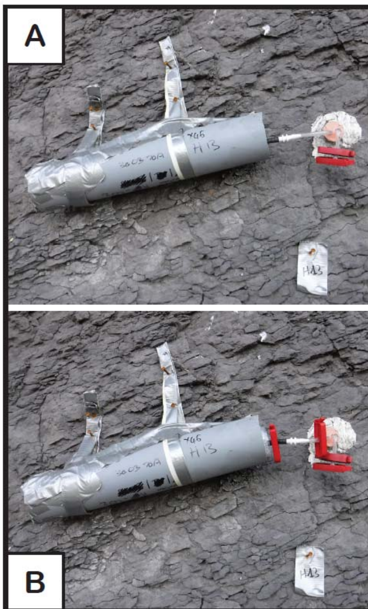
Figure 4: A: Zeolite molecular sieve connected to a chamber for passive CO 2 trapping. The zeolite molecular sieve is encased in the grey PVC tubing and connected for months to the chamber using a white connector. B: Zeolite molecular sieve ready to be disconnected from chamber. The red clips are positioned so that they seal both the zeolite molecular sieve and the chamber.
