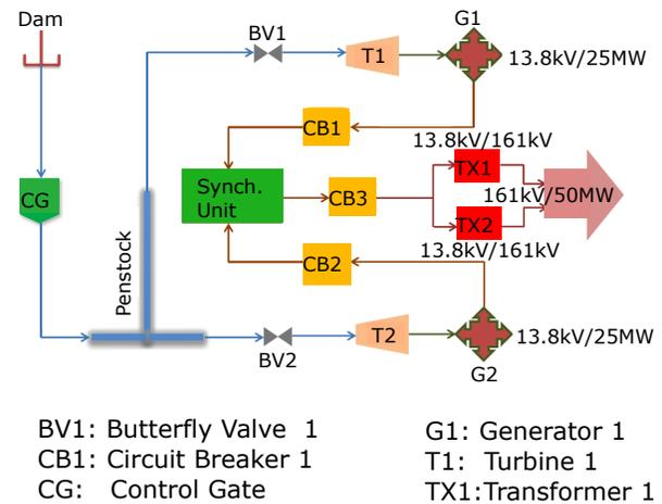
**Figure 7.** Schematic of a 50MW hydroelectric power plant.
