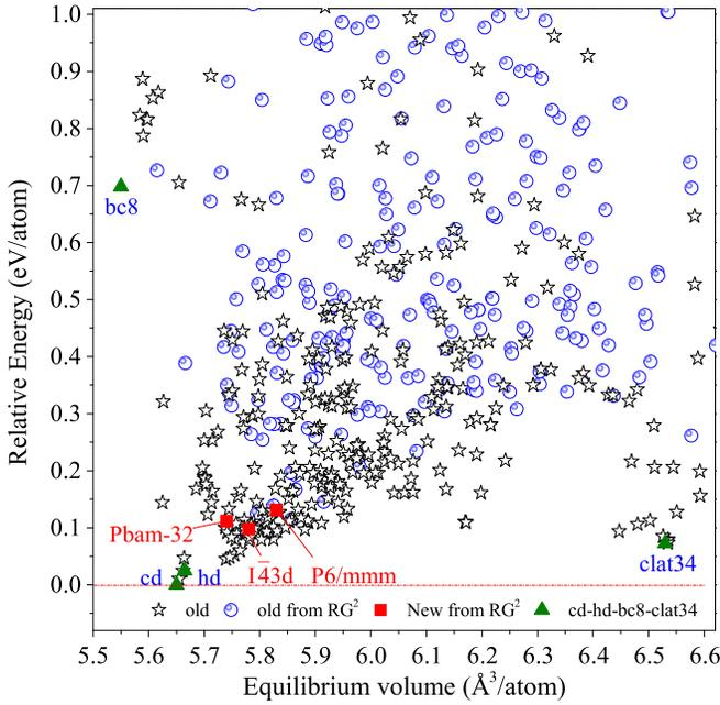
FIG. 2. Scatterplot of the PBE-based relative average energy (eV/atom) against equilibrium volume ( $\text{\AA}^3$ ) of the carbon version *Pbam-32*, *P6/mmm*, and *I43d* predicted in this work (red squares), the  $sp^3$  carbons previously predicted in the past decades [4] (black five-point stars), as well as those  $sp^3$  carbons discovered in our recent stochastic search [5] (blue circles). Some well-known carbon phases (green triangles) are also plotted in for comparison.
