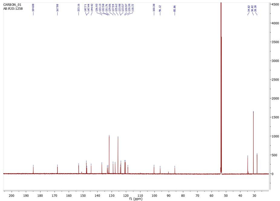
**Figure S36.**  $^{13}\text{C}$  NMR spectrum of **6** recorded in  $\text{CD}_2\text{Cl}_2$ .
