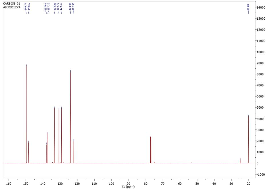
**Figure S6.**  $^{13}\text{C}$  NMR spectrum of 4-(4-bromo-2-methylphenyl)pyridine recorded in  $\text{CDCl}_3$ .
