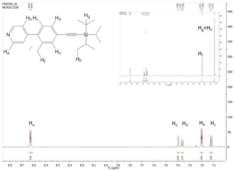
**Figure S11.**  $^1\text{H}$  NMR spectrum of 4-(2-methyl-4-((triisopropylsilyl)ethynyl)phenyl)pyridine recorded in  $\text{CDCl}_3$ .
