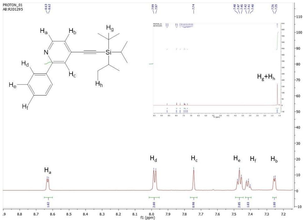
**Figure S17.**  $^1\text{H}$  NMR spectrum of  $\mathbf{L}^2\mathbf{H}$  recorded in  $\text{CDCl}_3$ .
