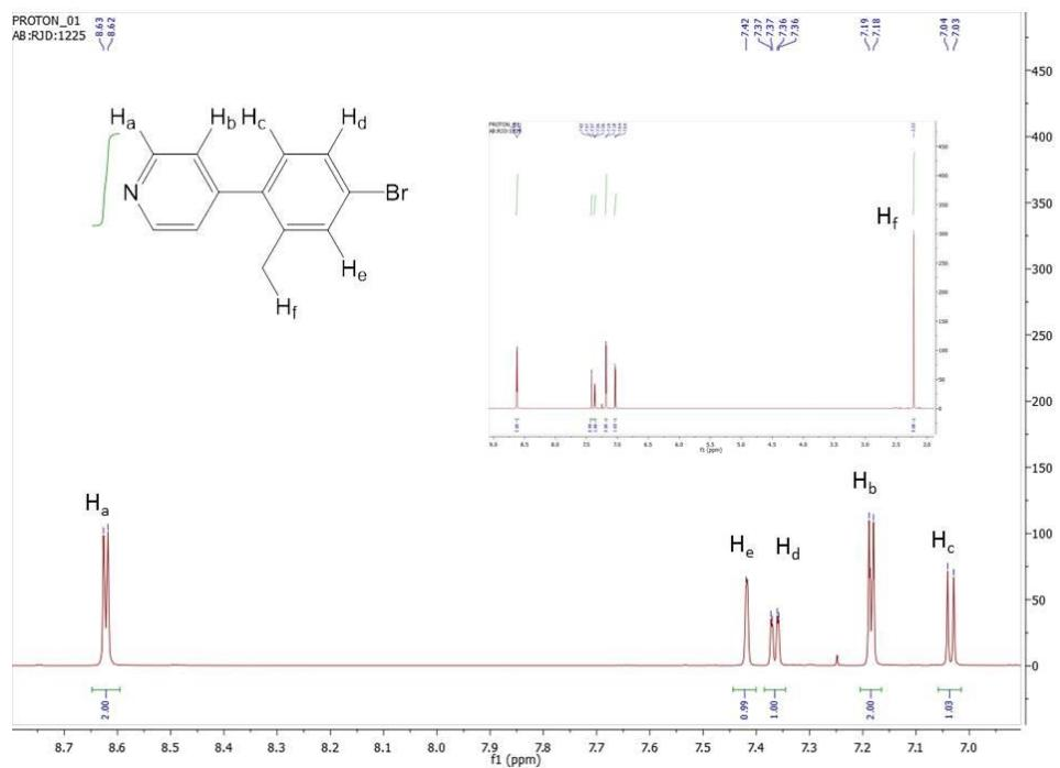
**Figure S5.**  $^1\text{H}$  NMR spectrum of 4-(4-bromo-2-methylphenyl)pyridine recorded in  $\text{CDCl}_3$ .
