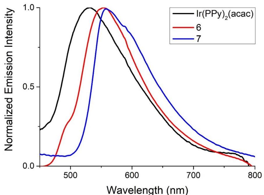
**Figure S54** Emission spectra of complexes  $\text{Ir}(\text{PPy})_2(\text{acac})$ , **6**, and **7** recorded in PBiBM films.
