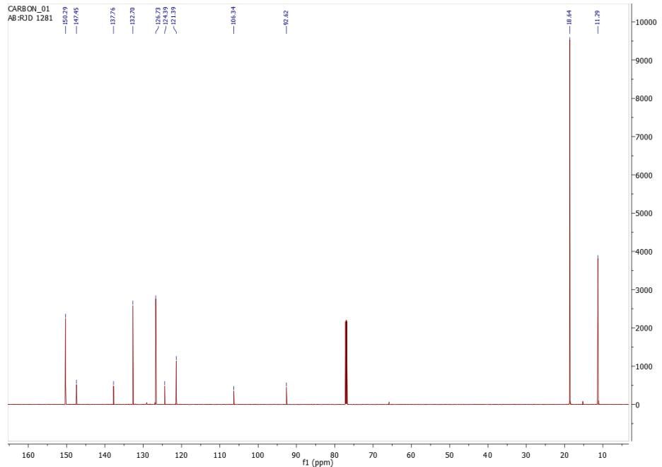
**Figure S10.**  $^{13}\text{C}$  NMR spectrum of 4-(4-((triisopropylsilyl)ethynyl)phenyl)pyridine recorded in  $\text{CDCl}_3$ .
