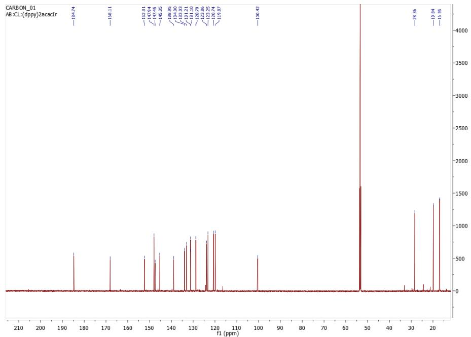
**Figure S26.**  $^{13}\text{C}$  NMR spectrum of **1** recorded in  $\text{CD}_2\text{Cl}_2$ .
