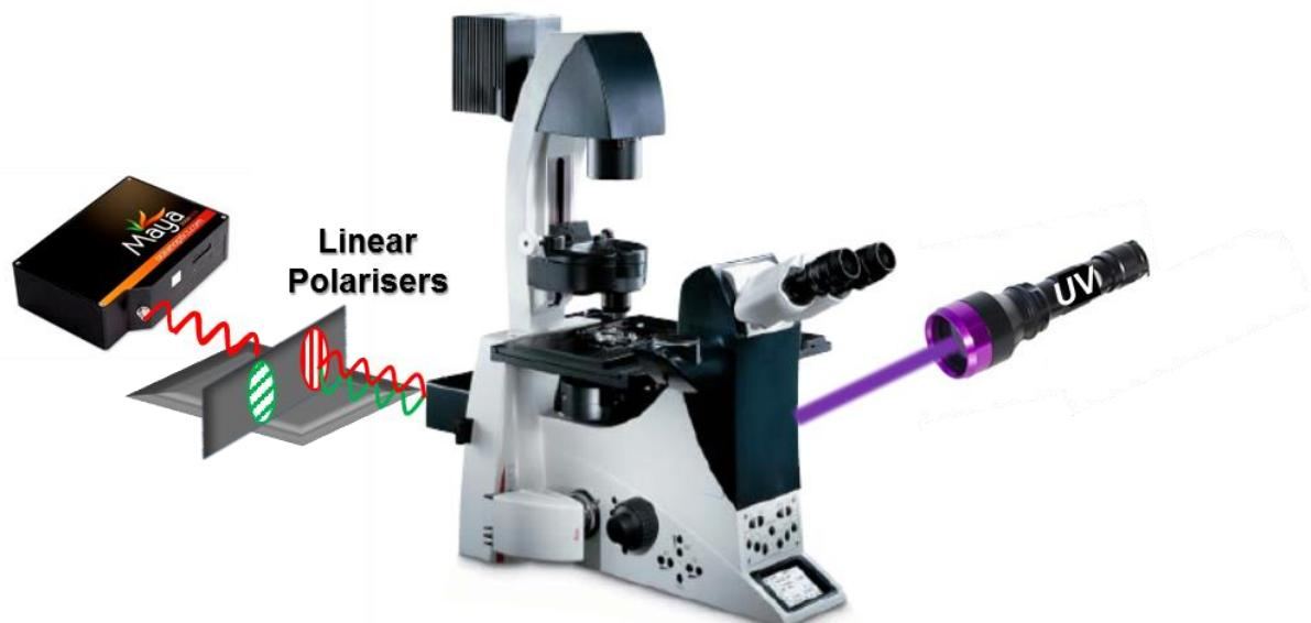
**Figure S59** Schematic diagram of the Polarisation Microscope used to determine PR (polarisation ratio).
