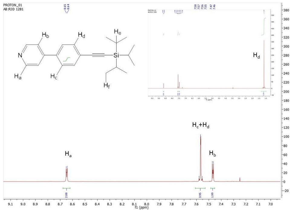
**Figure S9.**  $^1\text{H}$  NMR spectrum of 4-(4-((triisopropylsilyl)ethynyl)phenyl)pyridine recorded in  $\text{CDCl}_3$ .
