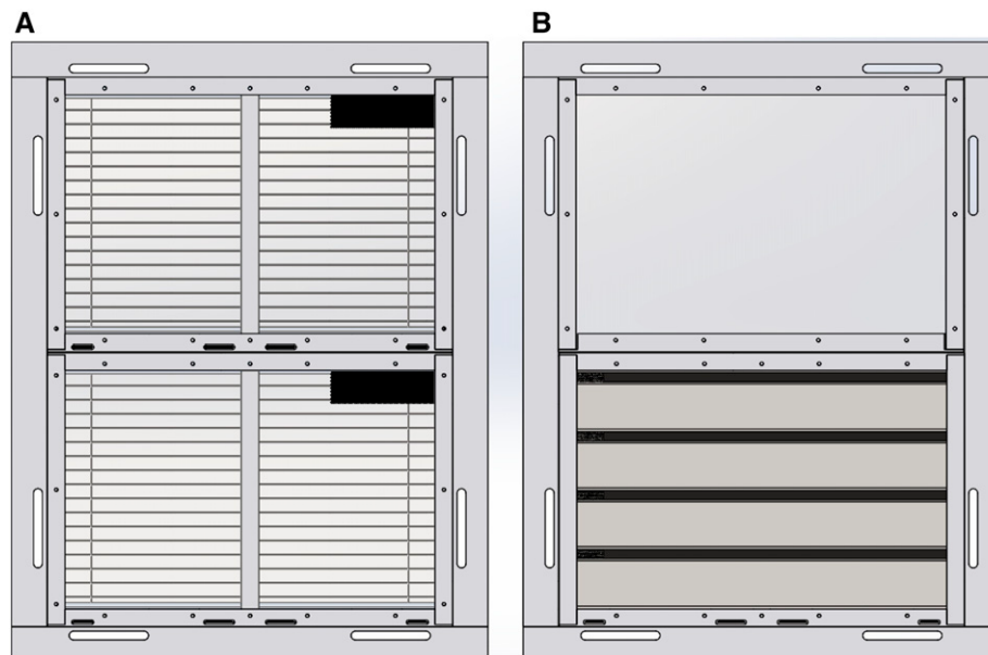
FIGURE 5. Prototype windows (internal view). Where A is the blinds window (W1) and B is a window combining an opaque panel at the top and concertinaed panel at the bottom (W2). This figure appears in color at www.ajtmh.org .
