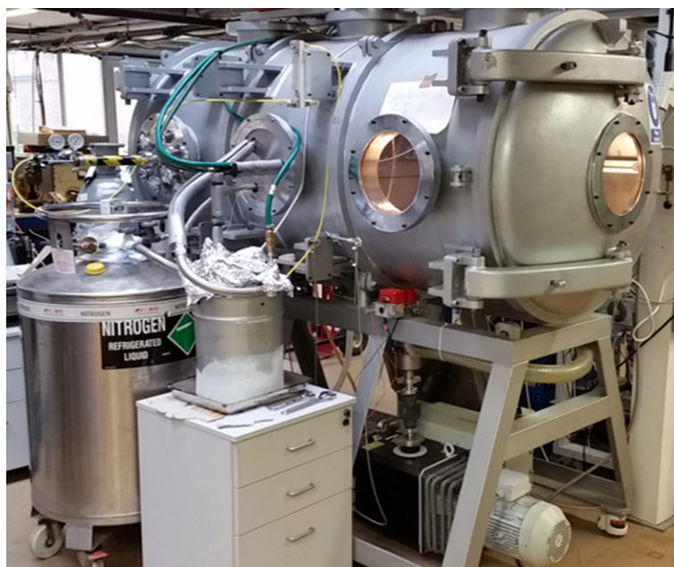
Fig. 2. The Large Mars Planetary Environmental Simulations Chamber (centre), vacuum pump (bottom), liquid nitrogen supply (left) and CO 2 gas cooler (front left of centre).
