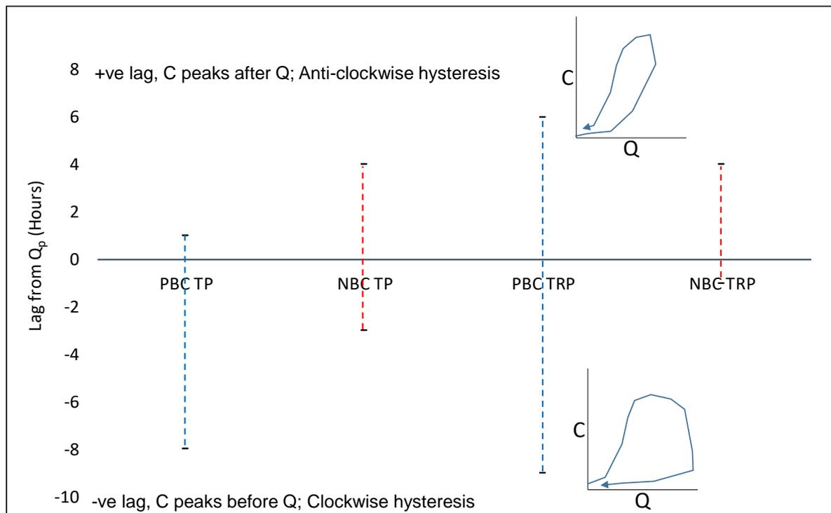
**Figure 5.** Plot showing the range of lag times for TP and TRP in NBC and PBC for all events. The lag times were calculated from the observed data from when the peak concentration (of TP and TRP) occurred relative to the time when  $Q_p$  occurred. Sketches of Q-C relationships during hysteresis loops are also shown for clockwise and anti-clockwise hysteresis.
