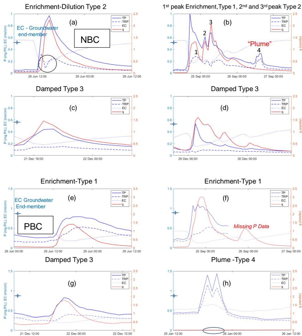
**Figure 3.** Time series plots of observed specific discharge ( $q$ ), Electrical Conductivity (EC) (note that the EC units are  $\text{mS cm}^{-1}$ ) and Total Phosphorus (TP) and Total Reactive Phosphorus (TRP) concentrations during events, indicating different event types. The first two rows (panes a-d) show four examples from the NBC; the last two rows (panes e-h) show four examples from the PBC. Specific discharge  $q$  is shown on the right-hand y axis.
