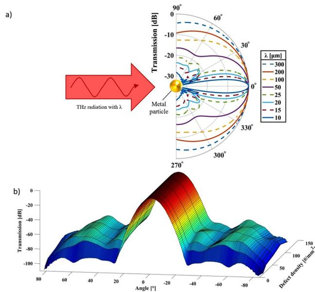
**Figure 3.** (a) The forward scattering of THz radiation with different wavelengths incident on a metallic sphere with a radius of  $20\ \mu\text{m}$  as predicted by the Mie theory (from FDTD simulation). (b) Simulation of the angular scattering pattern of a defect rich sample with different defect densities.
