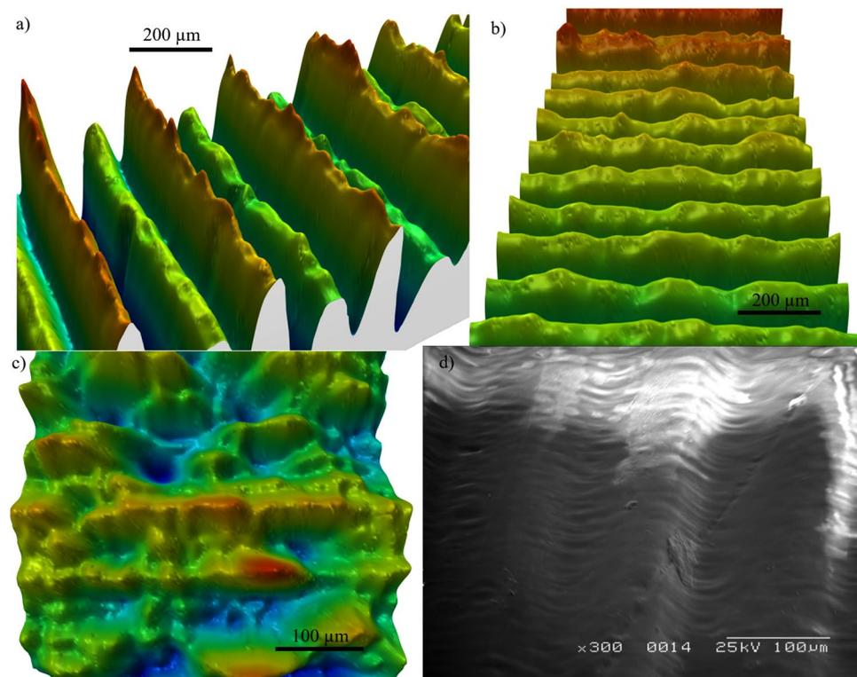
**Figure 2.** (a–c) 3D maps from the optical profilometer measurements. (a) shows the alternating height on sample 3. (b) shows the surface roughness on the top of the ridges. (c) while the presence of grooves on sample 4 is visible, the defects are in the same size order as the periodicity. (d) The micrograph of sample 4 on the other hand, gives the impression that there is a periodicity that could support the measured spoof THz SPPs.
