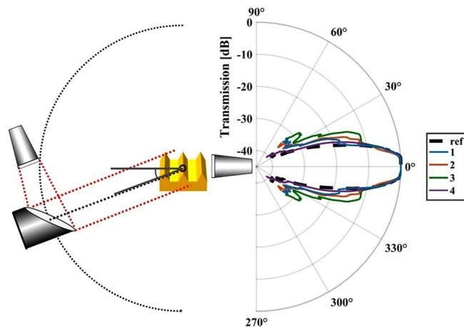
**Figure 4.** Schematic of the angular measurement setup (left) and the polar plot of the results (right). The angular plot shows the averaged intensity below the cut-off frequency of the individual samples. All SPP samples show an increased acceptance angle. Additionally, side lobes as they are known from Mie scattering are visible.
