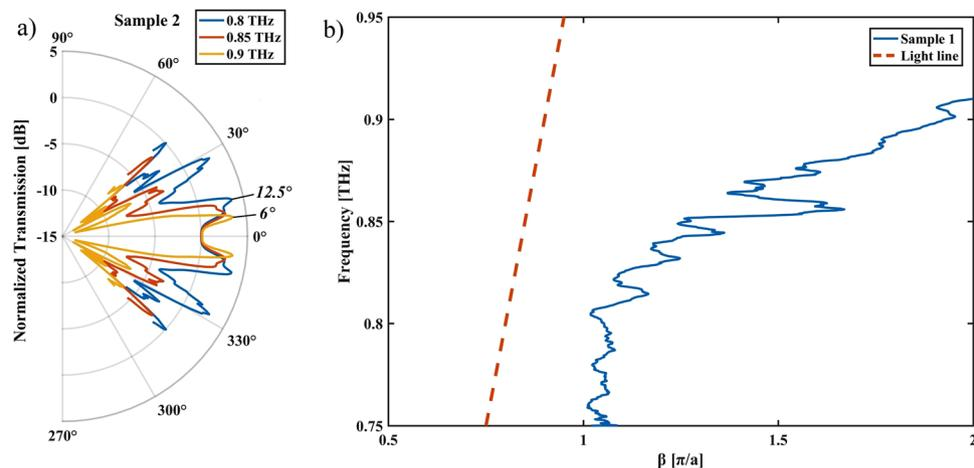
**Figure 5.** (a) Frequency resolved angular plots show that the scattering lobes move toward the forward direction with increasing frequency. Due to normalization with the bare horn antenna, the forward scattering lobe is removed. (b) The dispersion curve shows that the bound wavelength of the sample.
