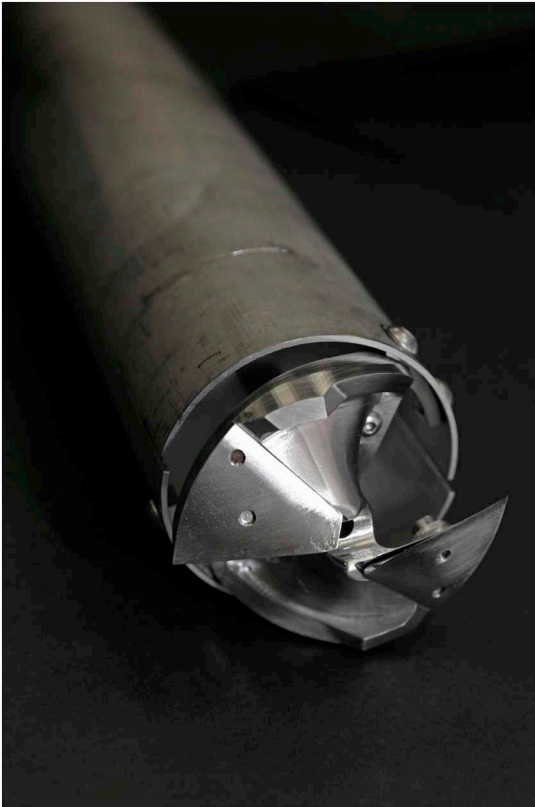
Fig. 2. RAID front end, with the ice cutters and rotary barrel visible. The system diameter is 80 mm.
