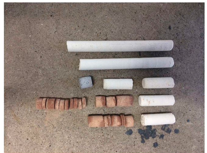
Fig. 12. Core samples obtained from tests in Hartham Park limestone (white cores), Locharbriggs sandstone (reddish cores) and microgabbro (grey core).
