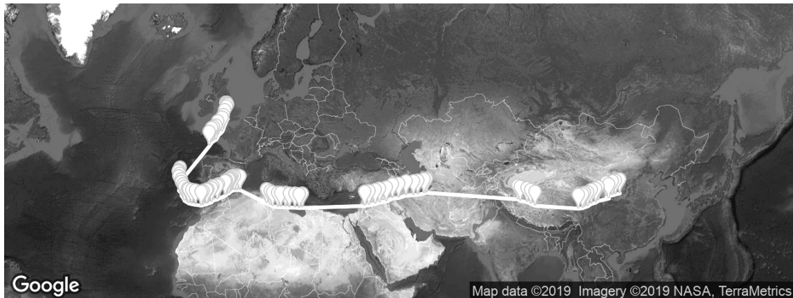
Figure 8. The flight path of the UBSEDS22 superpressure balloon, March 2017. During each valid telemetry burst, the Iridium Network determined the beacon's location by tracking its position in the satellite's service beams. Each location has a typical circular error probable of approximately 5km and is represented by a marker. The gaps between the markers show where the nighttime temperature caused the beacon to stop transmitting; the temperature above Morocco on the second night was sufficiently high to allow the beacon to continue transmitting.
