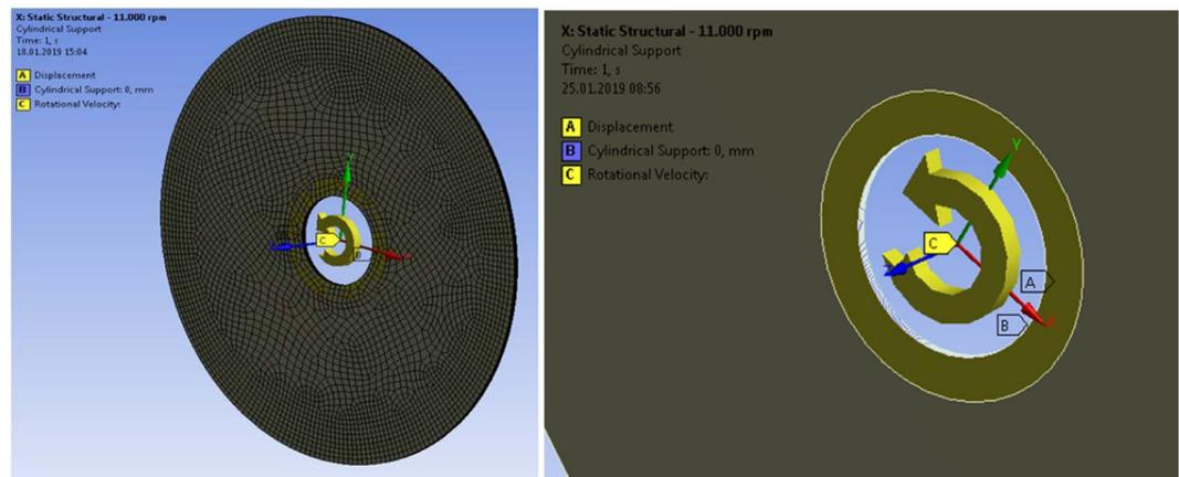
**Figure 14.** Orientation of the coordinate system and application of boundary conditions. 'A' indicates displacement in z-direction = 0, 'B' indicates cylindrical support in inner diameter and 'C' is Rotational Velocity of all bodies.
