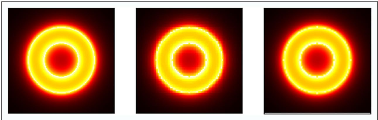
**Figure 2:** The magnitude of the magnetic field around a ring magnet, left,  $400 \times 400$  pixel finite-element analysis model, centre,  $40 \times 40$  pixel exported subset, right,  $400 \times 400$  pixel interpolation of the subset.
