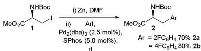
Scheme 1. Negishi cross-coupling in the synthesis of \alpha -amino acids, Jackson and co-workers [30].
