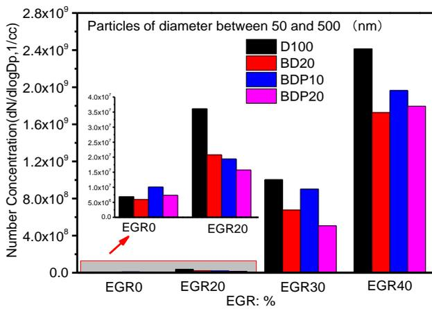
Fig. 9(c) Particle number concentration of the four different fuels varying the EGR rates (50 (nm) <diater<500 (nm) )
