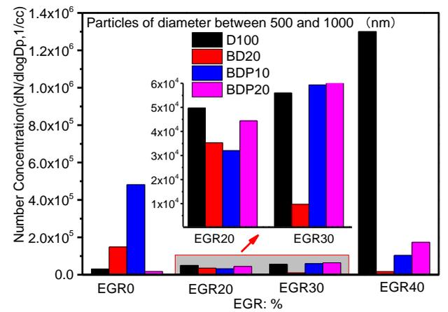
Fig. 9(d) Particle number concentration of the four different fuels varying the EGR rates (500 (nm) <diater<1000 (nm) )
