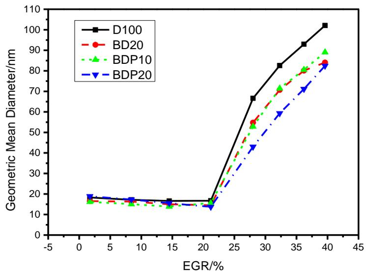
Fig.7. Geometric mean diameter of the four different fuels at varied EGR rates
