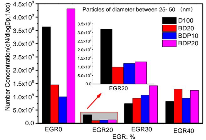
Fig. 9(b) Particle number concentration of different fuels varying the EGR rates(25(nm)<diater<50(nm))
