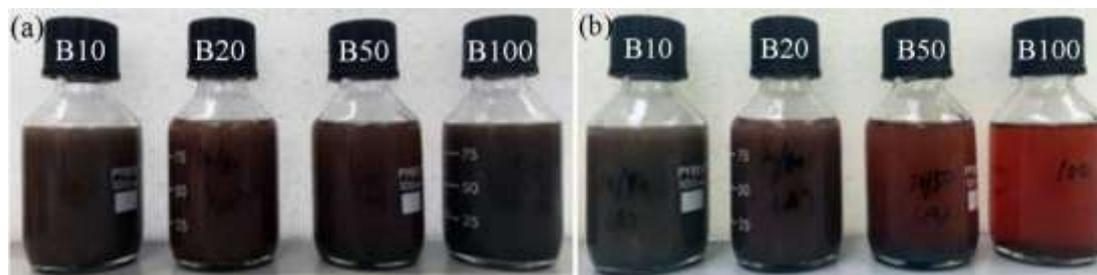
14 Fig. 3. Digital photographs of biodiesel-diesel suspension employing Al@C nanoparticles with various ratio of palm oil methyl ester.
